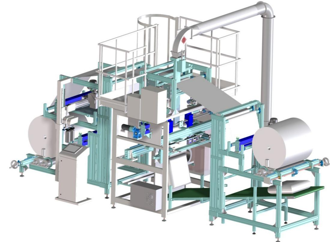
This **vertical version** has been specially designed to automatically manufacture finished cushions made **both of polyester microfibre and nonwoven polypropylene**.
